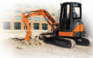
Compact excavator and ASV-style tracks are constructed of a unique rubber compound for superior ability to withstand abrasions, chips, and cuts.
