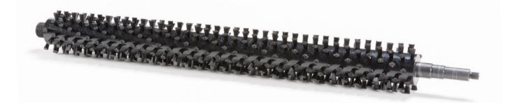
At John Deere, we're committed to providing hardworking, long-lasting parts for your operation. That's why we created our **DT Rotary Turf Brush**. Ideal for dense turf varieties of cool and warm season turf grasses, this rotary turf brush uses an exclusive helix design for bristle mounting. The helix design promotes improved striping and consistent cut quality while improving the ability to stand up the grass blades without increasing brush depth.
